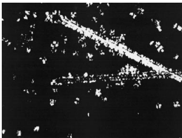
Fig. 8. PP crystallization in the presence of aramid fibres, at 408 K (7 min after reaching the sample crystallization temperature).
